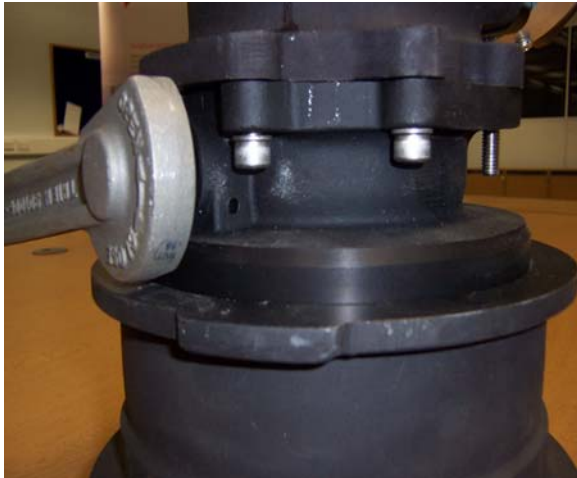
Coupler/Pressure controller re-assembled
